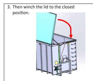
Remove the winch handle and place it back in its place.
