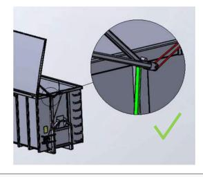
6. If, for any reason, the safety support does not automatically move to the safety position, push the lever towards the container.
